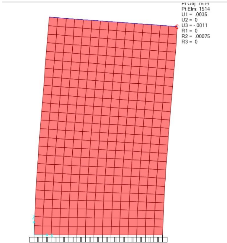
Figure 12. Deflection of wall 2 due to Eqx ultimate
