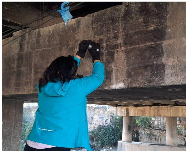
Figure 2. Rebound Hammer Test
