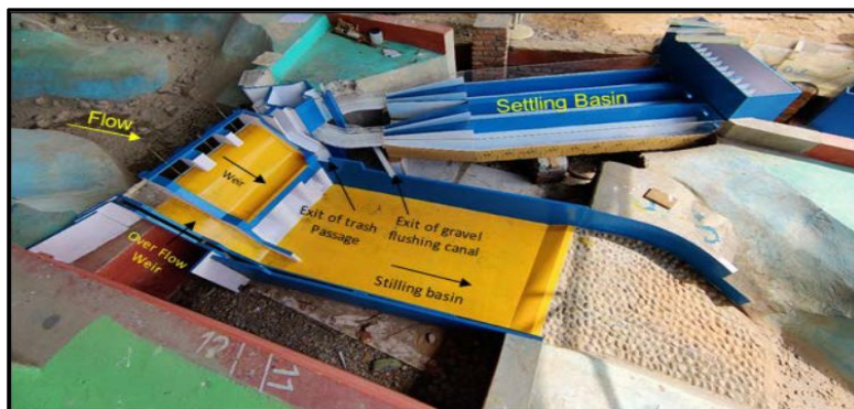
Figure 3. Arrangement of Physical Model of MMHPP (Scale 1:35)
