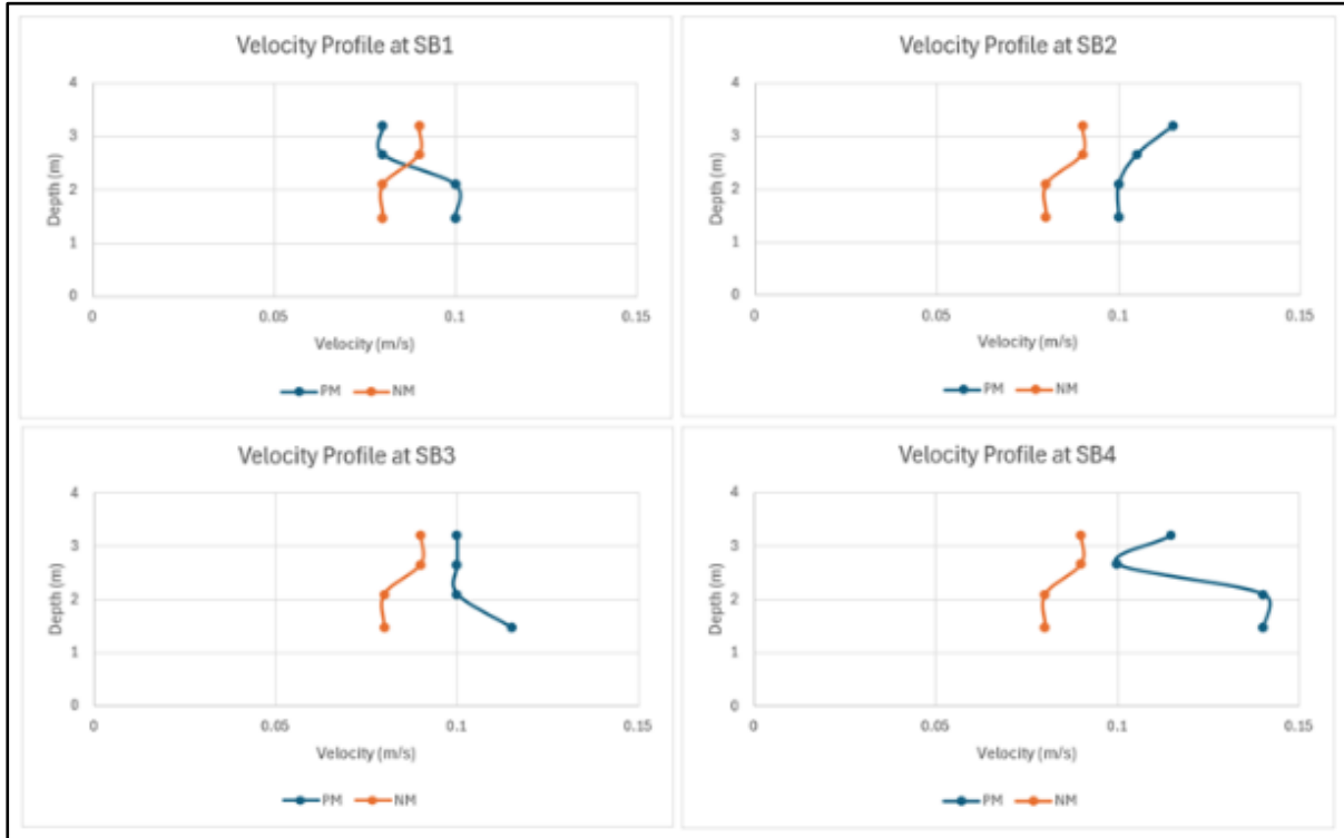
Figure 12. Comparison of velocity profile between Physical and Numerical model at 25m from inlet of settling basin
