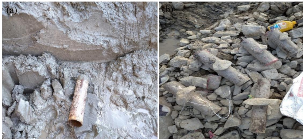
Figure 4. Soil sampling for consolidation test: (a) field sampling location, (b) collection of undisturbed soil samples
