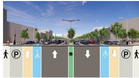
Figure 24: Perspective sectional view of 50m wide road (West side, Section at CC)
