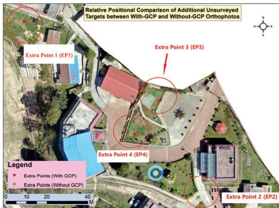
Figure 6. Relative positional comparison of additional points between the with-GCP and without-GCP orthophotos Table 7. Relative positional differences of additional unsurveyed targets between the with-GCP and without-GCP orthophotos
