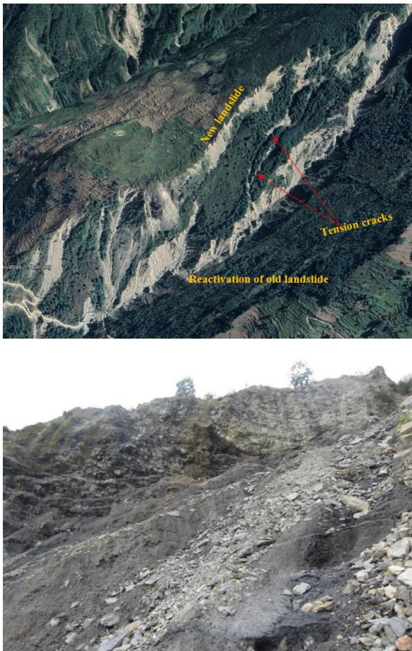
Fig. 8: (a) Typical morphology of the landslide illustrating origination of new landslide, reactivation of old landslide and new cracks around the area and (b) Rock exposure at middle section of the landslide.
