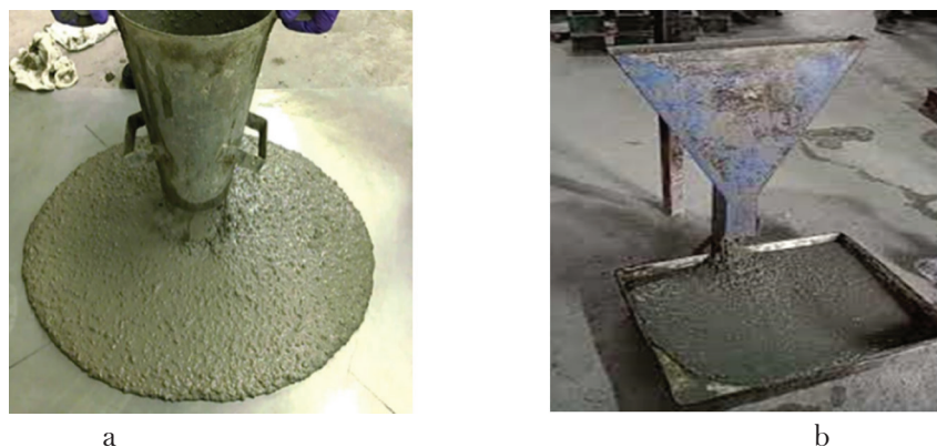
Figure 2: Fresh property test a) Slump test b) V-funnel test
