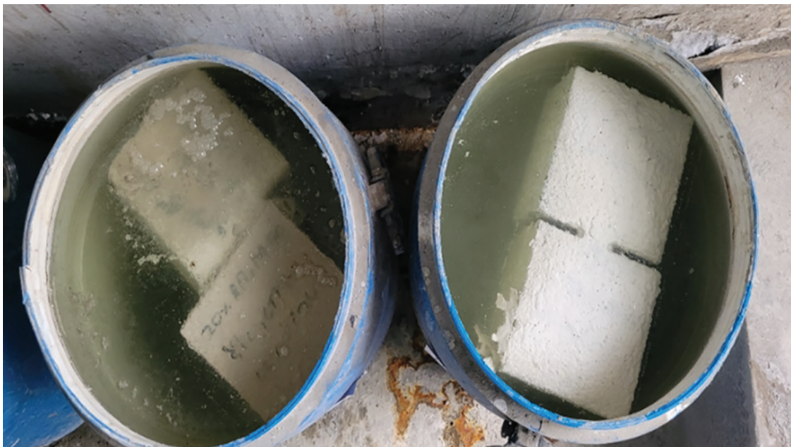
Figure 6: Durability test acid curing
