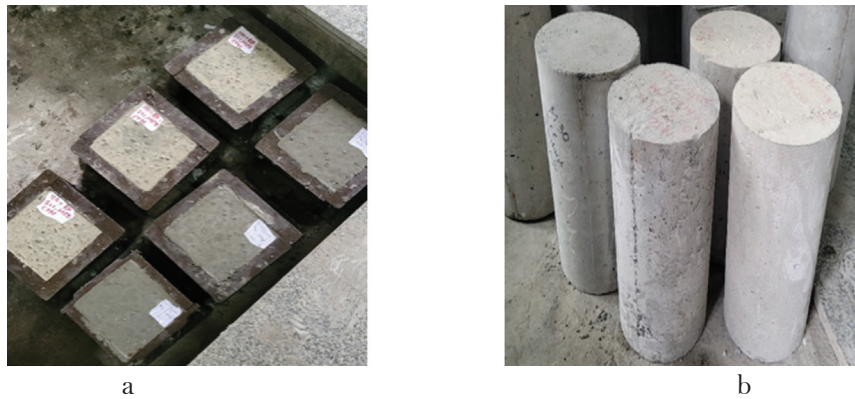
Figure 3: Concrete samples a) Cubical 150x150x150mm b) Cylindrical 300x150mm
