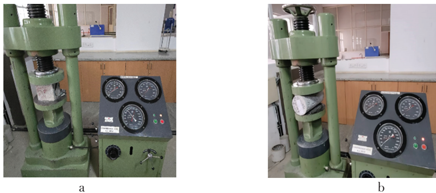
Figure 4: Hardened tests a) Compressive strength tests b) Split tensile strength test
