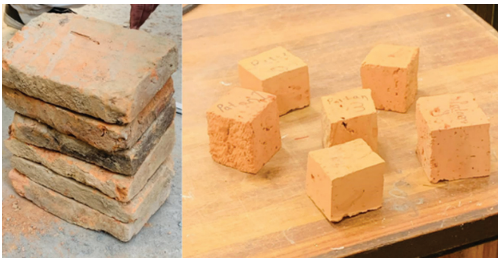
Figure 10: Original brick samples (left, stacked) and prepared 40 mm cube specimens (right) for uniaxial compressive strength testing.
