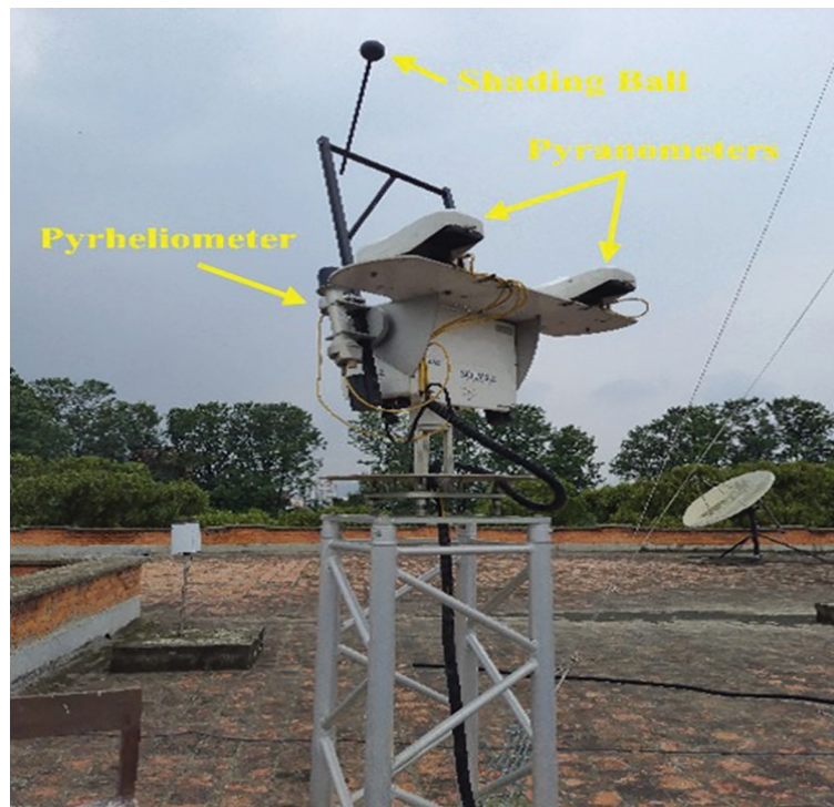
Figure 1: 2D-Solsys2 solar tracker mounted with the sensors
