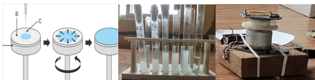
Fig. 2. (a) Spin coating technique (Akhtar et al.,2015), (b) Aluminium added ZnO solution b) Spin coater.
