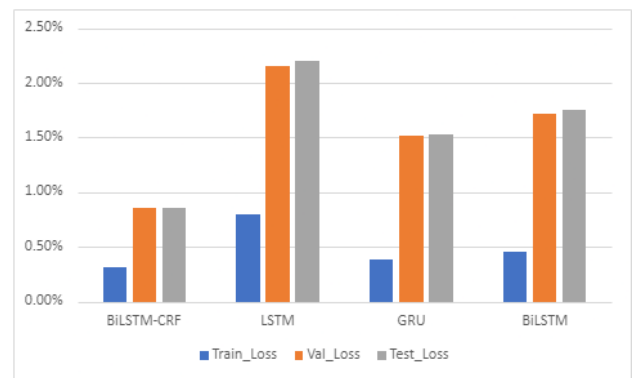
Fig. 11. Comparison between BiLSTM-CRF with Word2Vec and established models GRU, LSTM, and BiLSTM based on Train_Loss, Val_Loss and Test_Loss
