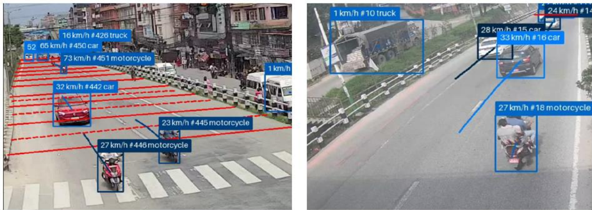
Figure 3: Video output after using YOLO and Open CV libraries
