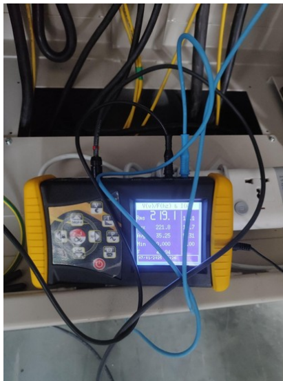
Figure 3. Power analyzer connected at point of common coupling
