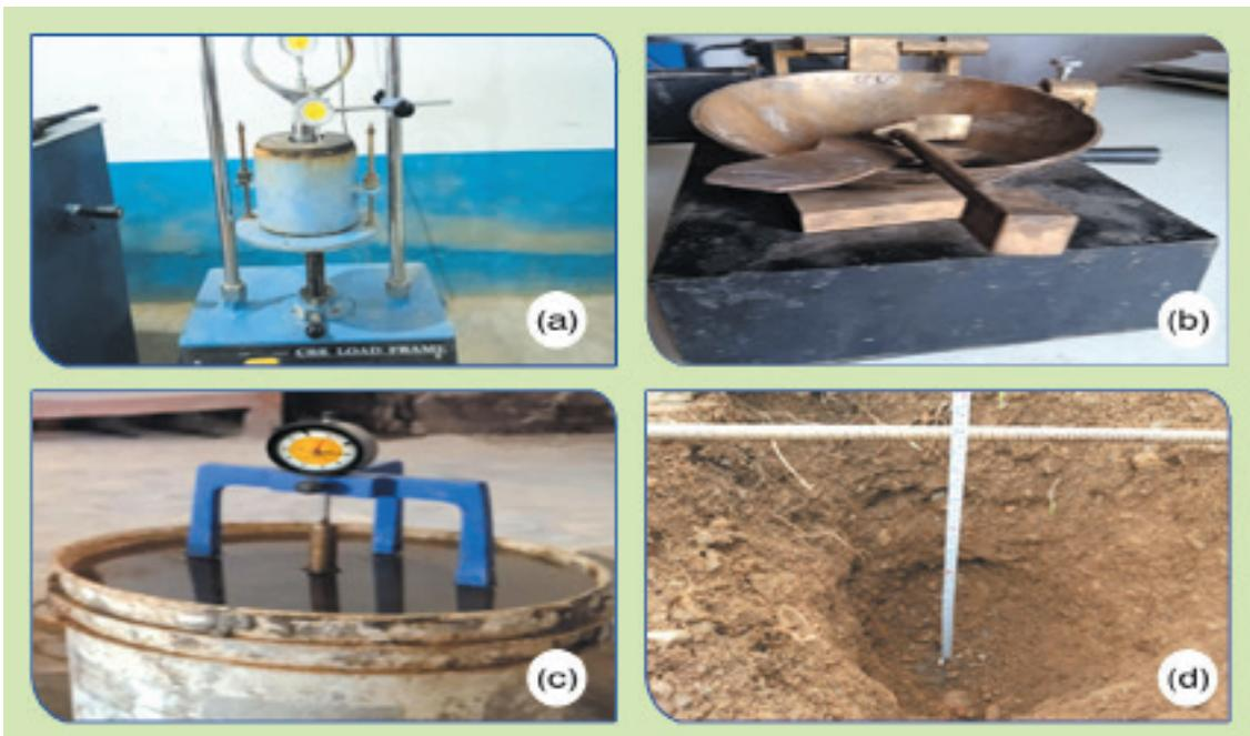
**Figure 1: Sampling and Testing. (a) CBR testing of samples, (b) Casagrande testing devices, (c) Soaking of Sample, (d) Sample taking from site,**
