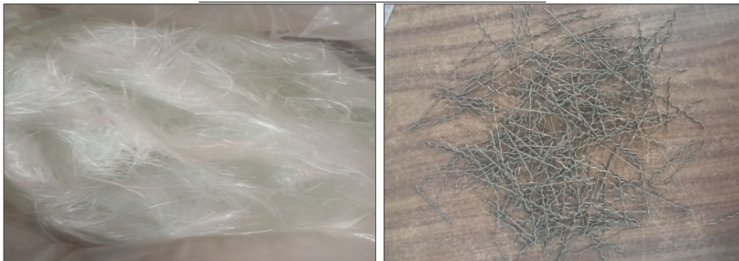
Figure 1 E- Glass fibers and corrugated steel fiber
