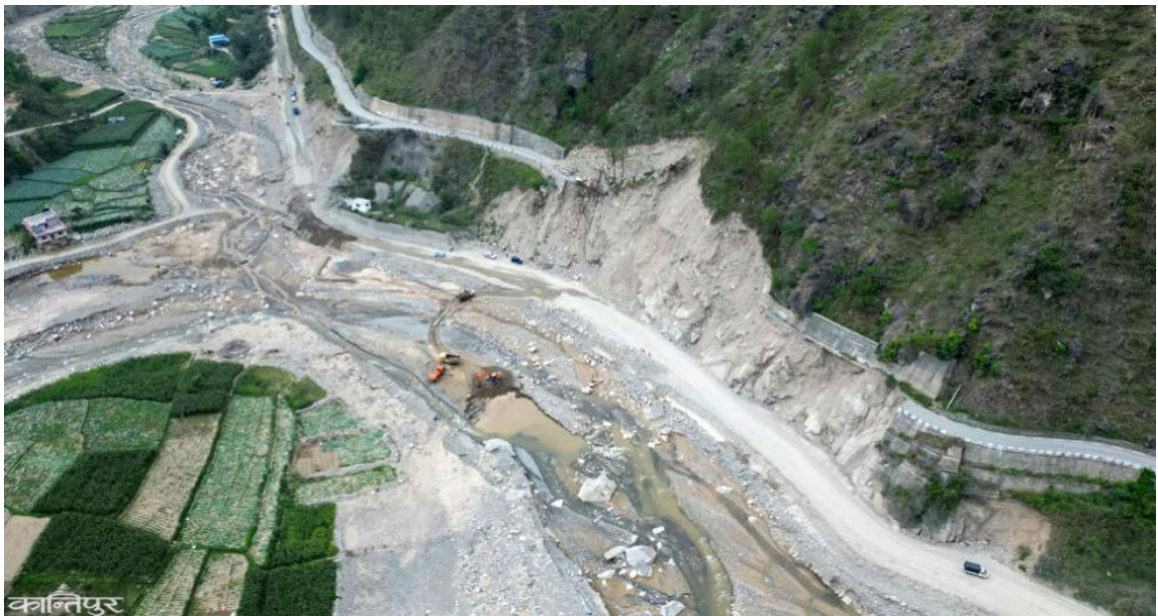
Figure 18 Damage caused by the Roshi river at Nepalthok on BP Highway (Source: https://ekantipur.com )
