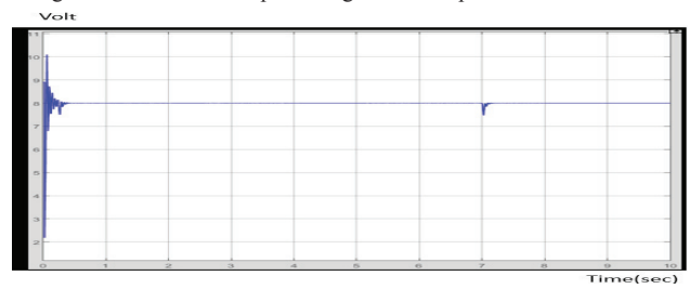
Fig. 11 Peak value of output voltage with a step load increased at 7 sec
