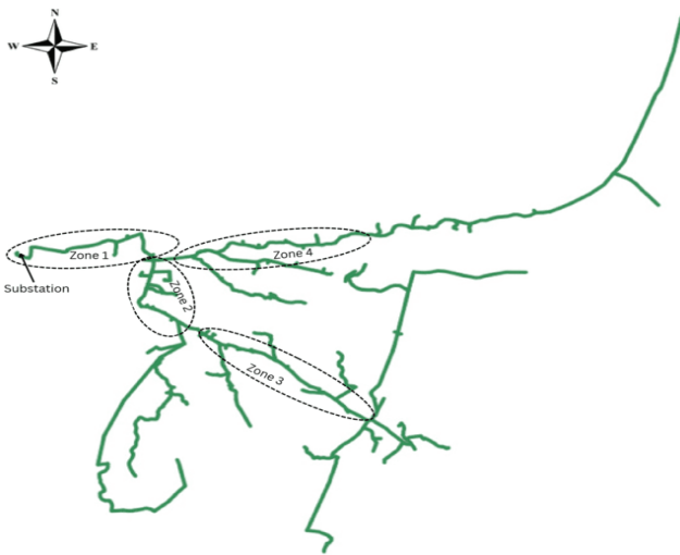
Fig. 8. 11 kV lines of the distribution feeder
