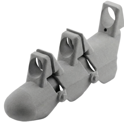
Fig 4. Hall-effect sensor and magnet mounting mechanism on a finger joint
