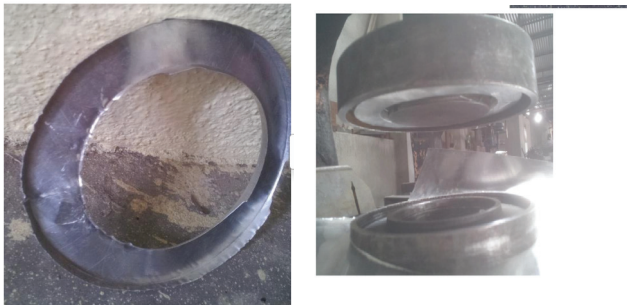
Figure 5. sheared flange of pleat base and pleat base stuck in the die
