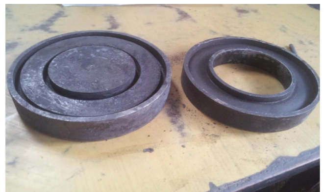
Figure 4. Heat treatment of dies for surface hardening
