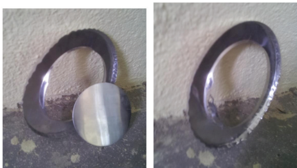
Figure 6. Non uniformity of flange still produced
