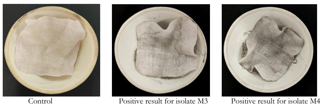
Figure 12 Application of pigment on cotton fabrics extracted from the isolates M3 and M4 using oatmeal agar medium
