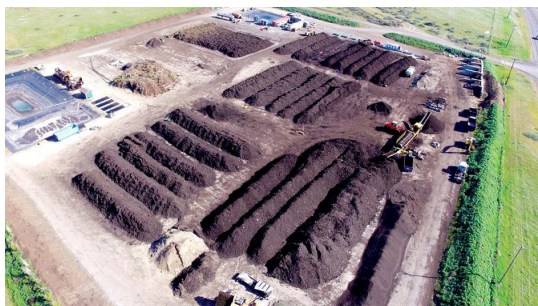
Figure 4. Windrow composting facility in Virginia (Coker, 2022)
